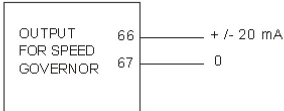
If necessary, the current outputs can be converted to voltage using a resistor across the terminals (250  $\Omega$  will convert the +/-20 mA into +/-5V DC).
