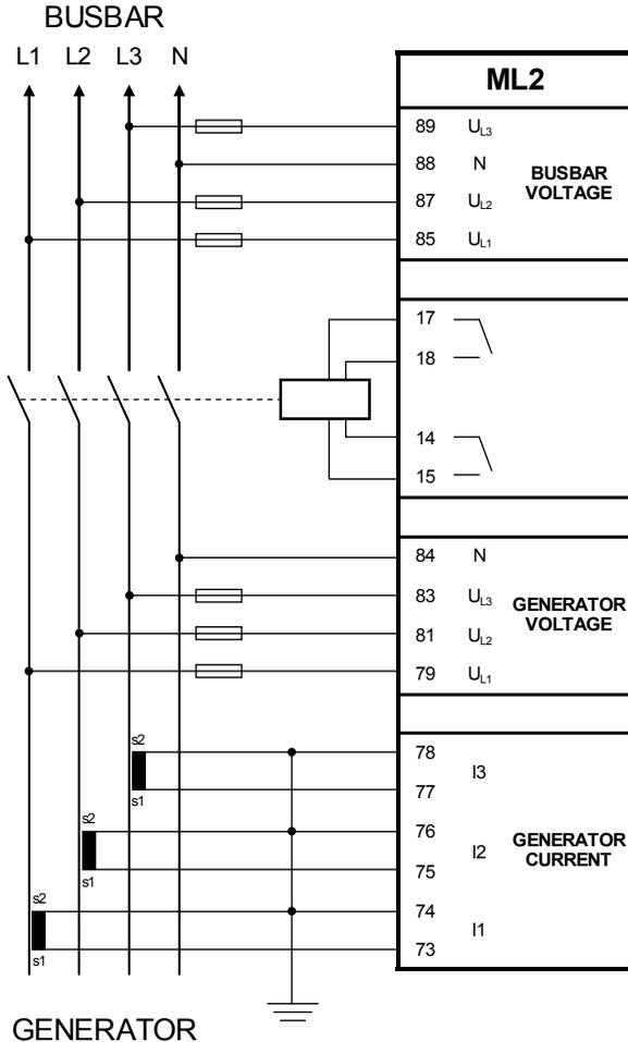
The neutral line (N) connection is not necessary for correct measurement. 3-phase without neutral is also possible. The current transformer ground connection can be on the s1 or s2 connection, whichever is preferred. Fuses: 2 A slow-blow.
