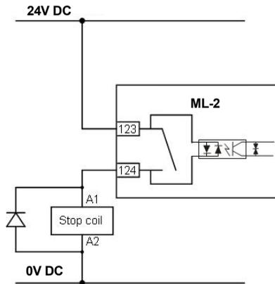
To avoid faulty activation of the stop coil caused by the wire break circuit, use a stop coil with the following specifications:
