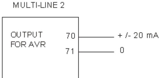
If necessary, the current outputs can be converted to voltage using a resistor across the terminals (250  $\Omega$  will convert the +/-20 mA into +/-5V DC).
