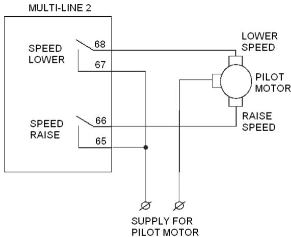
In order to extend the lifetime of the internal relays and prevent unwanted switching noise, it is recommended to use free wheel diodes (1N4007) if a DC voltage is used for the regulation. If an AC voltage is used for the regulation, it is recommended to use a varistor. The diode/varistor must be placed across the terminals of the pilot motor/external regulation relay coil.
