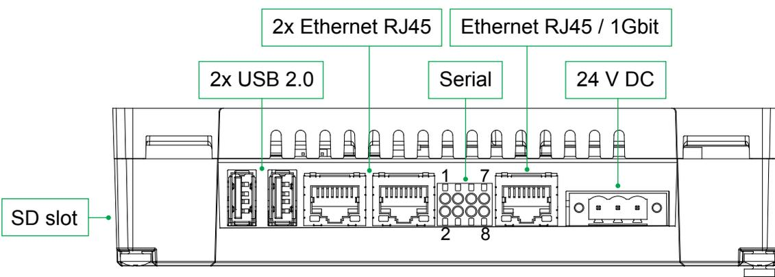
Connections that place a high data transfer load on the controller (for example, a SCADA system) should be connected to the controller through a switch.
