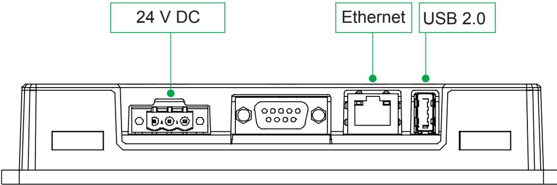
The TDU 107 Core can be connected to the controller directly or using a switch. Use a USB type A-B cable to connect a service computer to the AGC-4 controller if the TDU Core is connected directly to the controller.
