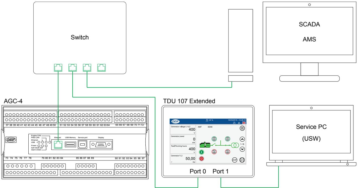
In system configurations without a high data transfer connection it is possible to connect the TDU 107 Extended version directly to the controller and connect a service PC to the TDU 107.
