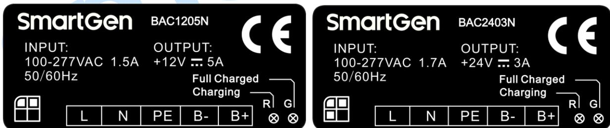
**Fig.2 – BAC1205N (left) & BAC2403N (right) Panel Drawings**
