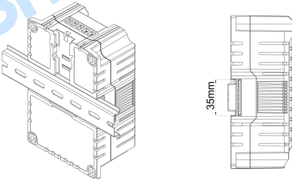
**Fig.4 – Guide-rail Installation**
