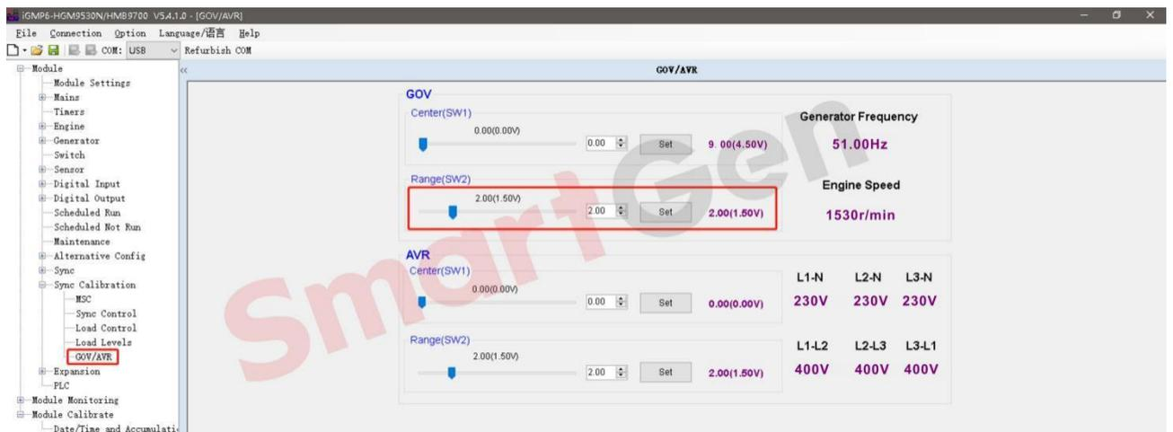
**Fig.76 Adjust SW2 of GOV at rated frequency of 51HZ**
