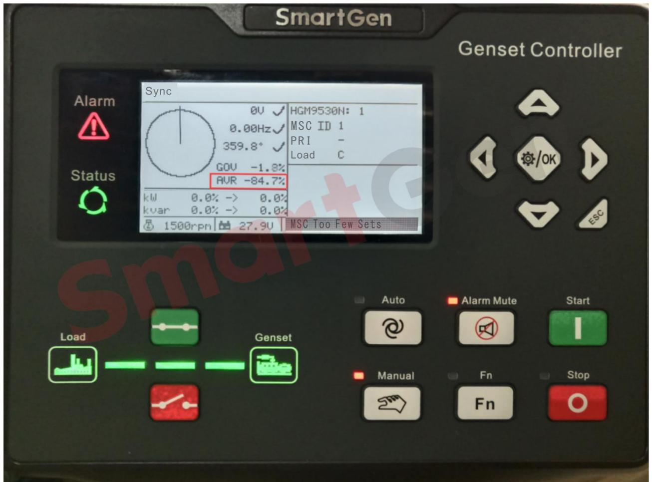
Fig.87 AVR output percentage at rated voltage of 220V
