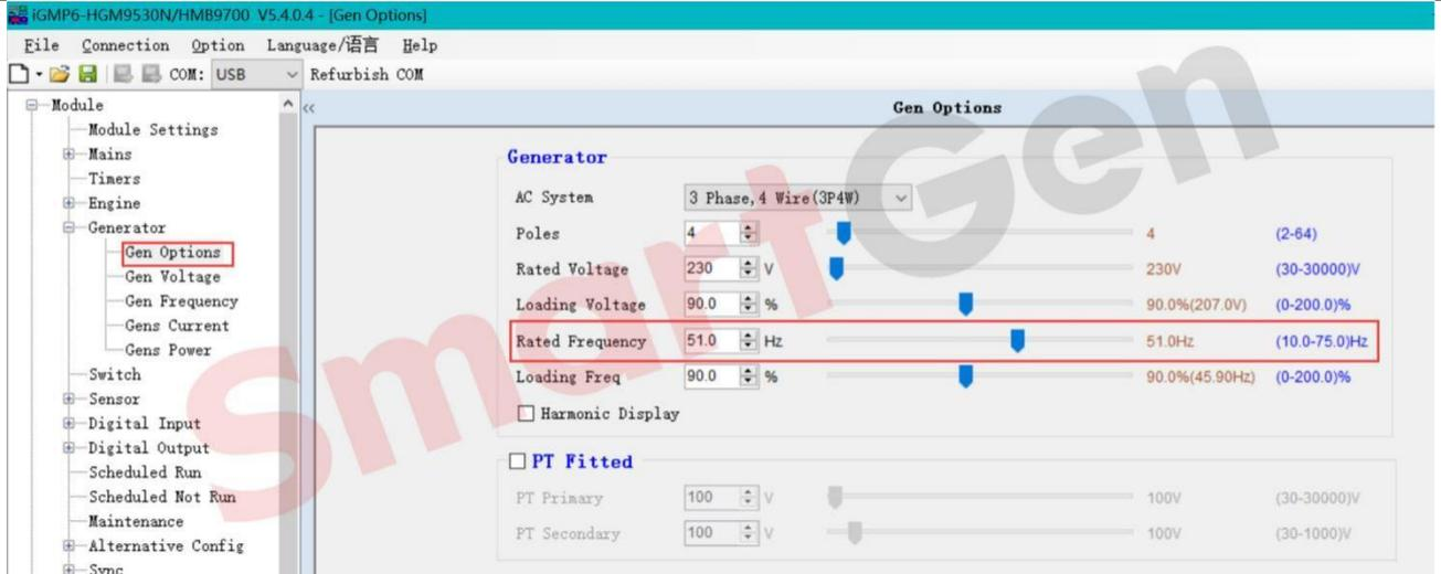
**Fig.74 Set the rated frequency to 51HZ**
