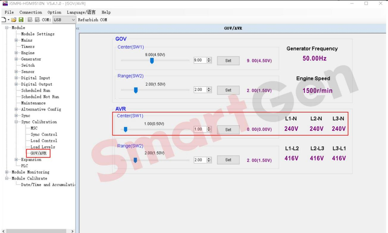
**Fig.85 SW1 of AVR at rated voltage of 240V**
