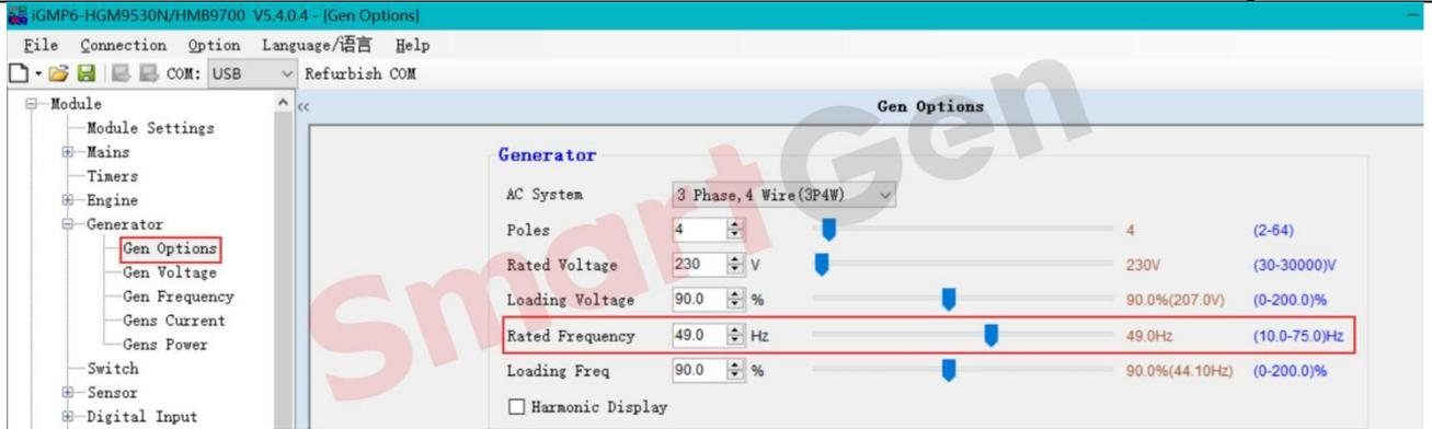
**Fig.77 Set the rated frequency to 49HZ**
