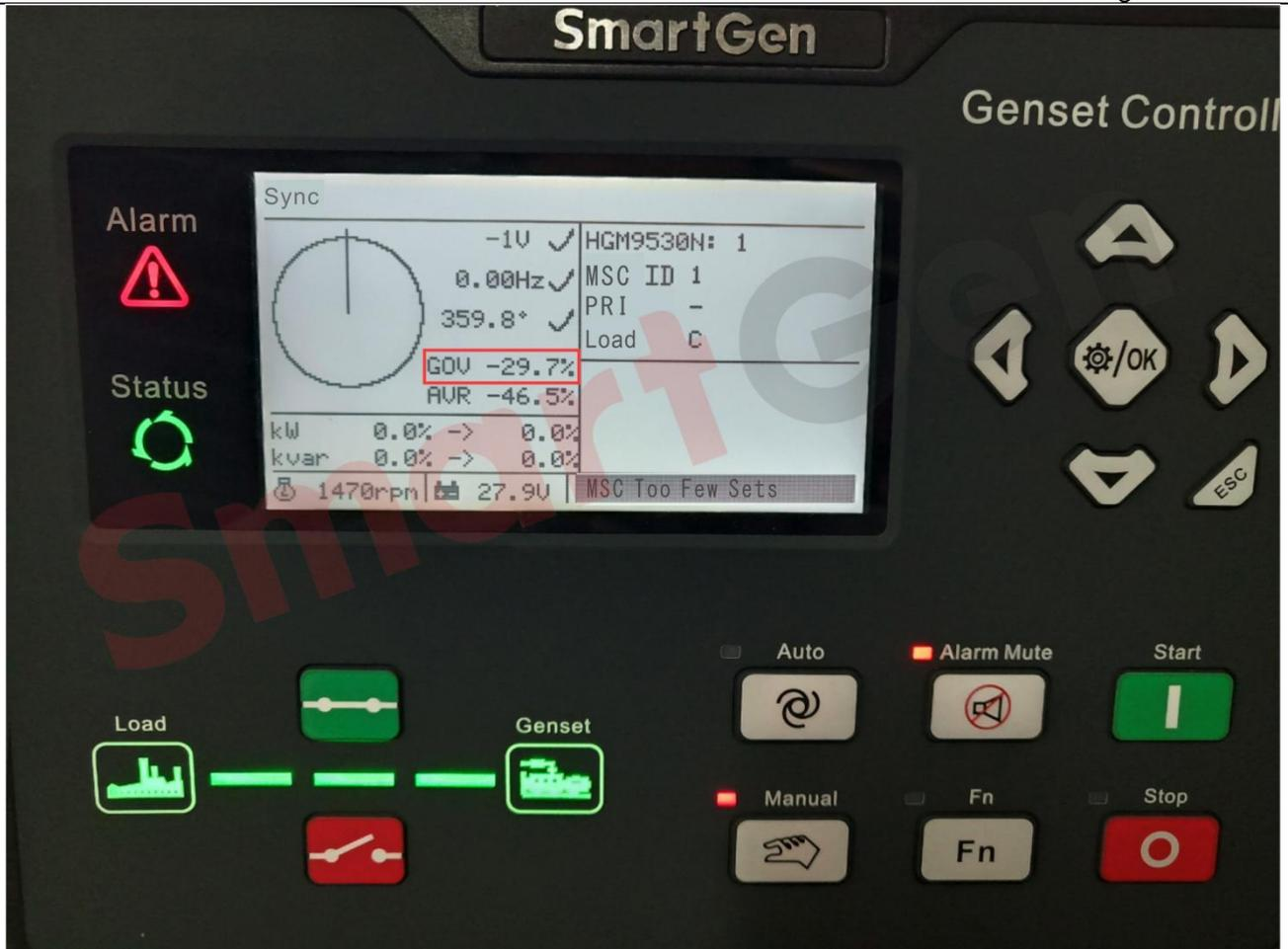
**Fig.78 GOV output percentage at rated frequency 49HZ**
