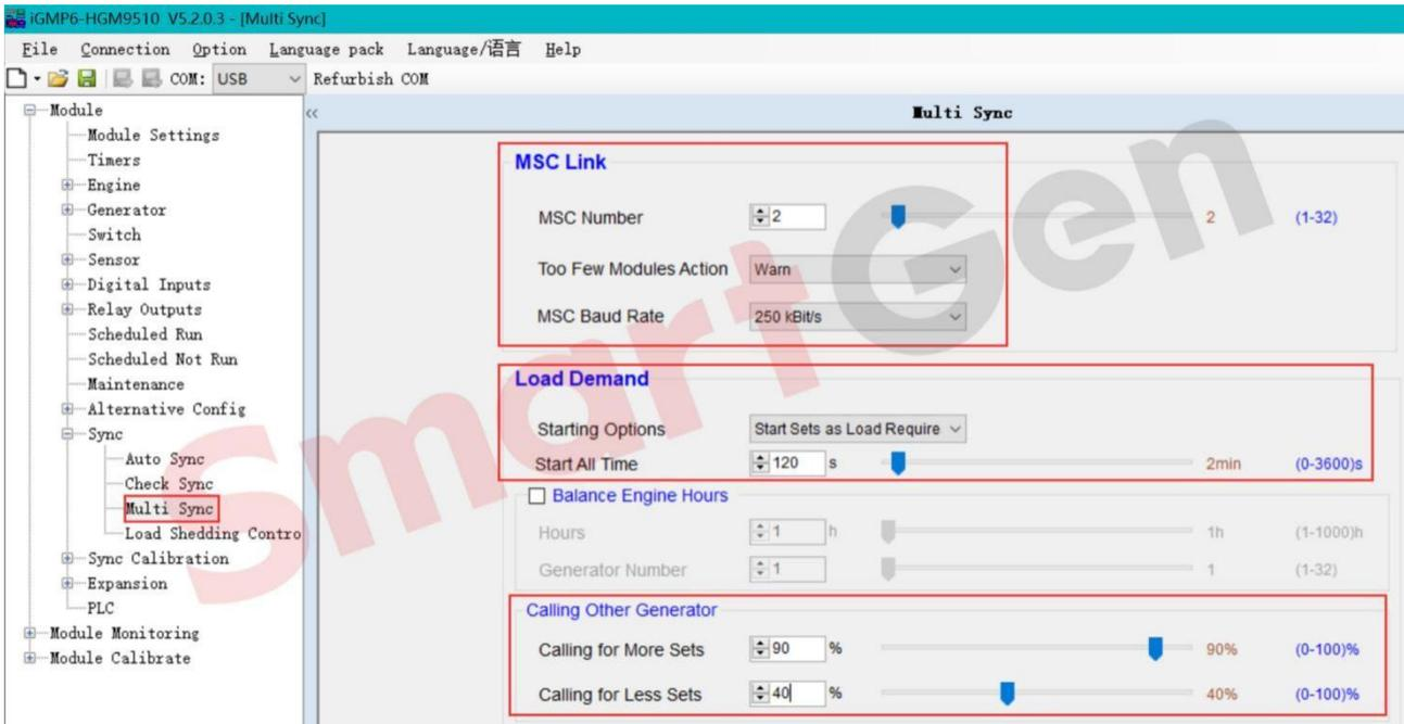
Fig. 57 Start Sets as Load Requires Setting
