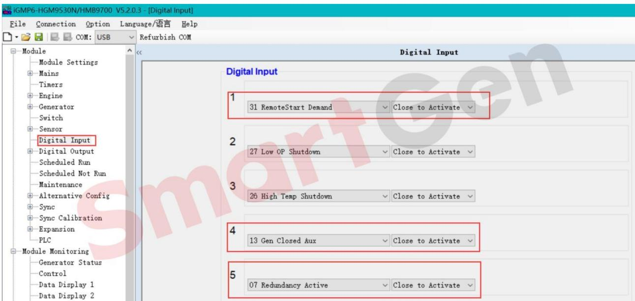
Fig. 50 HGM9530N Redundancy Mode Digital Inputs Setting
